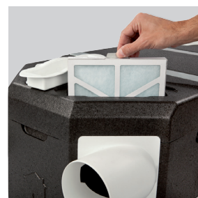
G4 filter (ISO coarse 65%, at 210 m 3 /h) and M5 (ISO ePM10 50%, at 210 m 3 /h). Easy access to G4 and F5 filters.
