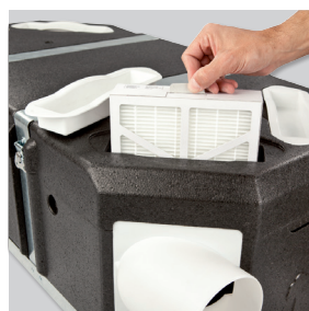
G4 filter (ISO coarse 65%, at 210 m 3 /h) and M5 (ISO ePM10 50%, at 210 m 3 /h). Easy access to G4 and F5 filters.
